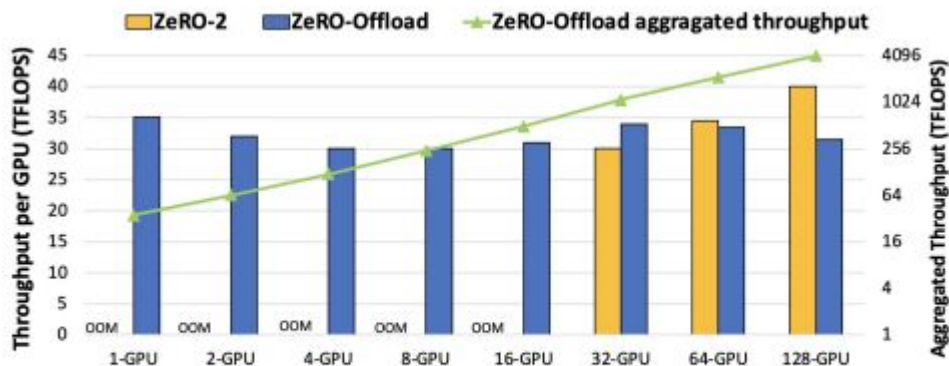
Figure 11: Comparison of training throughput between ZeRO-Offload and ZeRO-2 using 1–128 GPUs for a 10B parameter GPT2.
